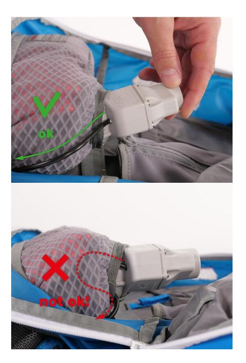
The area in which the black cable exits the deployment unit should be clearly visible. The Bowden cable should also feed into the shoulder strap without any significant bending. If this is the case, then the product has been installed correctly and your airbag is ready for use once the cartridge has been screwed in. If the cable is not clearly visible (as shown in the illustration on the right) and there is significant bending, please fix the problem as follows:
