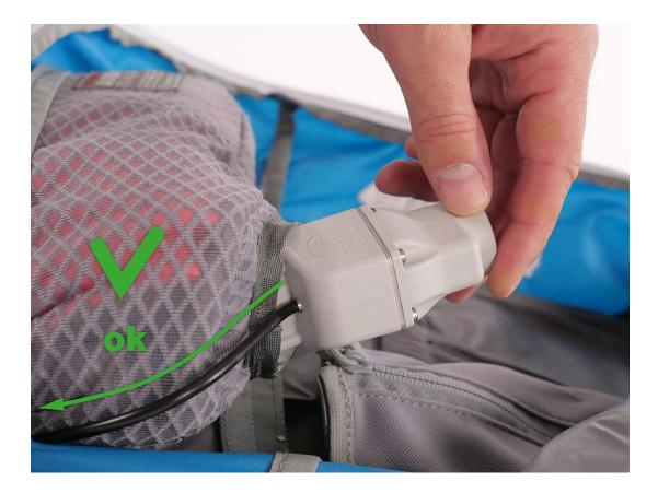
You can check that it has been correctly installed by conducting a training deployment. Please use the Trigger Test Tool supplied and follow the steps described in Chapter 5.5 of the manual delivered with the product. Please conduct the training deployment twice.
